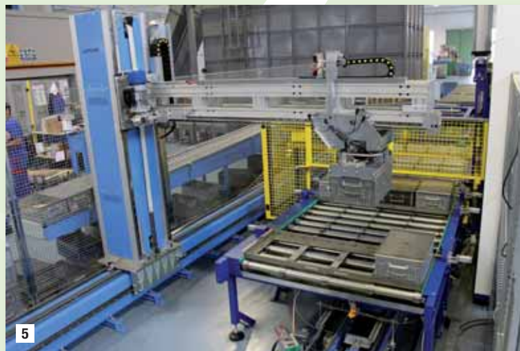
5 The two washing machines are supported by a robotic arm which collects the baskets coming from the loading zone. Depending on the information stored in the chip placed on every basket, the system interfaces with the two washing machines software allowing the regulation of the washing cycle needed for the components contained.
