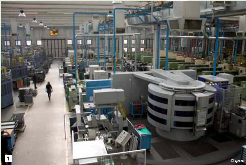
1 A bird's eye view of the Metal Work plant in Concesio (BS). The diversity of the materials processed involves a diversification of the work centres: in the foreground, a new generation transfer machining centre.
