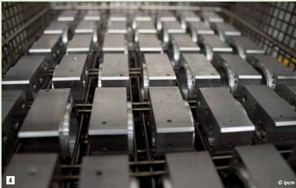
4 A close up of the fastening system for the most delicate components inside the basket to be inserted in the cleaning plant: The components are blocked in such a way that the movement of the container will not damage them. The plant designed by IFP Europe enables to choose the motion of the basket within the cleaning chamber: Rotary or tilting, depending on the characteristics of the product.
