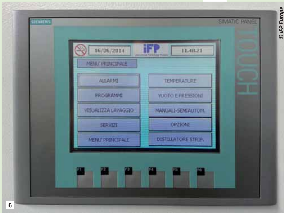
The PLC that simplifies the management and maintenance operations of the IFP system.
