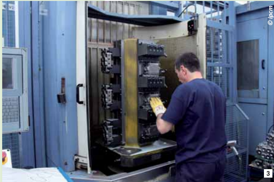
3 For the machining of its castings, Galtech employs highly efficient numerical control machines.
